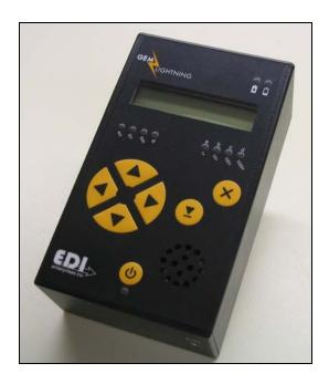
The BERT testing function can generate and detect pseudorandom and repeating bit patterns. It is used to test and stress data communication links, and it is capable of generating and detecting the following patterns:
